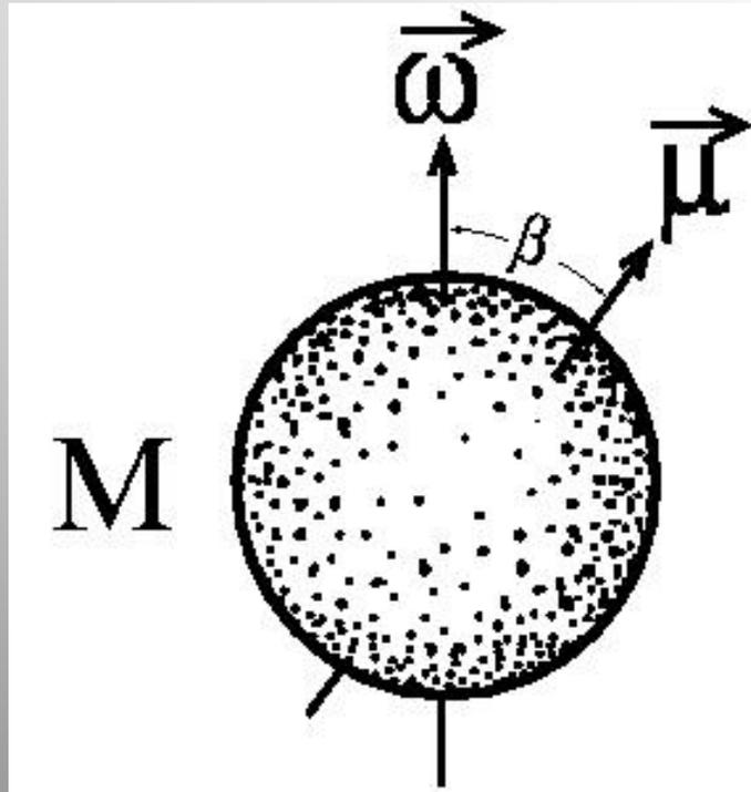
$$L_m = \frac{2}{3} \frac{\mu^2 \omega^4}{c^3} \sin^2 \beta = \kappa_t \frac{\mu^2}{R_t^3} \omega,$$
