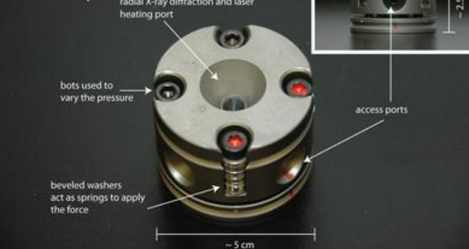
Diamond Anvil Cell Assembly
