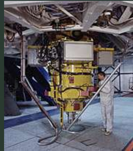
SPHERE - Spectro-Polarimetric High-contrast Exoplanet REsearch instrument
