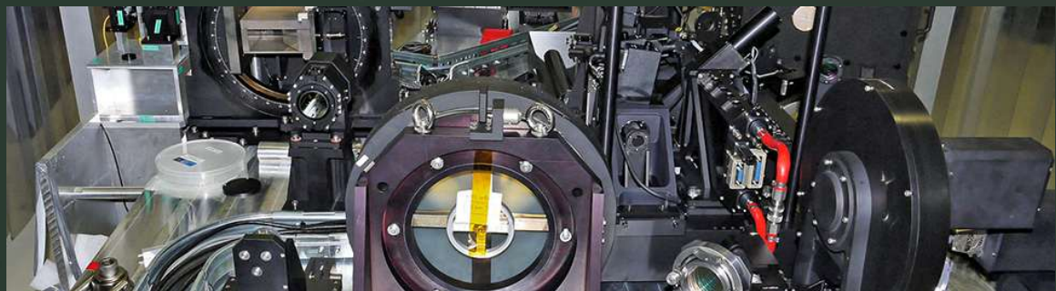
SPHERE - Spectro-Polarimetric High-contrast Exoplanet REsearch instrument
